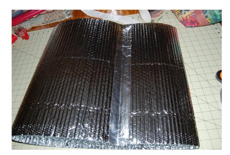
Butt the cut ends of the Reflectix® together and tape together with the shiny duct tape.
